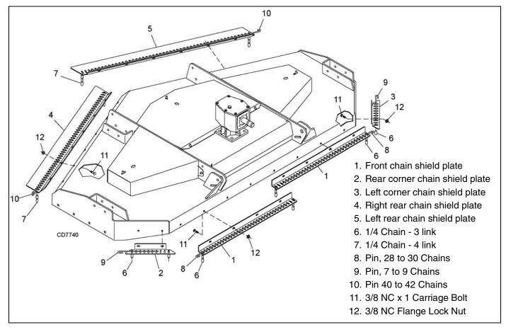
Figure 31. Chain Shield Installation
